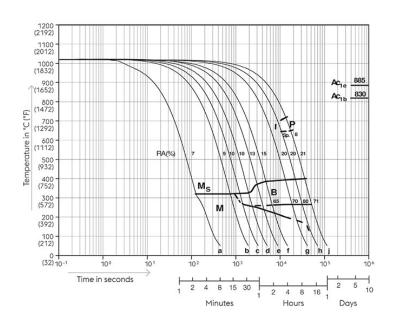
Austenitising temperature: 1020°C (1868°F) Holding time: 15 minutes 5...100 phase percentages 0.5...180 cooling parameter, i.e. duration of cooling from 800 - 500°C (1472-932°F) in s x 10<sup>-2</sup>
