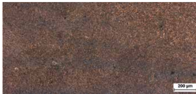
BÖHLER M303 EXTRA Homogeneous structure
